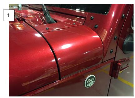
Wash the cowl with soap and water. Allow the cowl and surrounding areas time to dry. \*\*Recommended: Wipe the cowl with isopropyl alcohol to ensure the cleanest surface possible.
