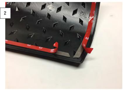
Familiarize yourself with how the cowl vent fits prior to peeling off the double sided tape. Then remove the tape and apply firm even pressure to ensure proper adhesion.
