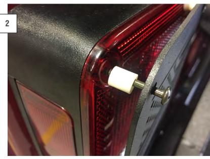
Place the supplied spacers between the tail light and the tail light guard. Secure the guard the vehicle using the supplied screws. The inner screws are the thinner screws.
