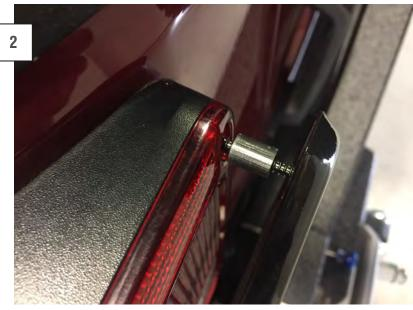
Place the supplied spacers between the tail light and the tail light guard. Secure the guard the vehicle using the supplied screws.
