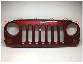
**Step 1\\**Using a panel removal tool, remove the (6) push clips holding the grille cover to the vehicle. Unplug the turn signals and pull the grille cover from the vehicle.
