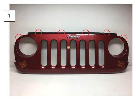
Using a panel removal tool, remove the (6) push clips holding the grille cover to the vehicle. Unplug the turn signals and pull the grille cover from the vehicle.
