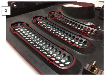
Press the insert into the grille cover ensuring that the insert clips onto the back edge of the grille. Install all (7) inserts and then reinstall the grille in reverse order.
