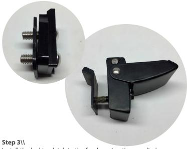
Install the locking latch to the fender using the supplied 13mm lock nut. Install the rubber isolator between the latch and fender. Install the hood latch using the supplied 10mm nuts. Install the rubber isolator between the latch and the hood.
