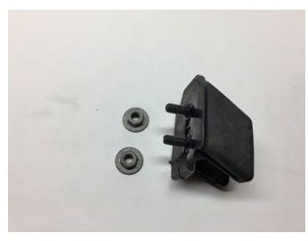
**Step 2\\**Prop the hood open and remove the (2) 10mm nuts that hold the hood latch to the hood, remove the latch from the vehicle.
