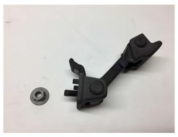
**Step 1\\**Begin by unlatching the factory hood latch. Gain access, and remove the 13mm nut that holds the hood strap to the fender.
