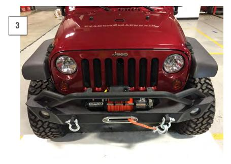
Reinstall the grille using the factory push clips.
