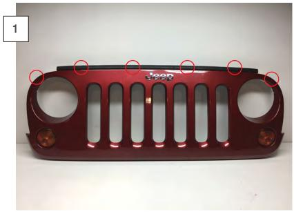
Using a panel removal tool, remove the (6) push clips holding the grille cover to the vehicle. Unplug the turn signals and pull the grille cover from the vehicle.
