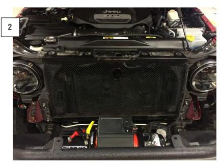
Place the grille insert onto the radiator support. It will be sandwiched between the radiator support and the factory grille and then secured using the factory push clips.
