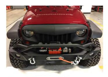
**Step 4\\**Reinstall the grille using the factory push clips.
