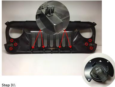
Press on the (4) supplied retaining clips. Install the turn signals into the provided brackets and then secure the brackets the grille using the supplied screws. Using the factory grille as a reference, apply the supplied weather stripping across the top of the grille.
