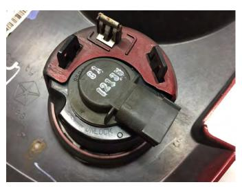
**Step 2\\**Remove the factory turn signals by unclipping them from the factory grille. Transfer them to the new grille.
