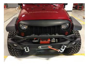
**Step 4\\**Reinstall the grille using the factory push clips.
