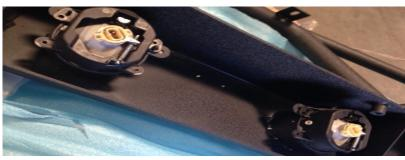
2) Locate the mounting plates and studs on the inside of the bumper. Also locate the 8 nuts and lock washers provided with
