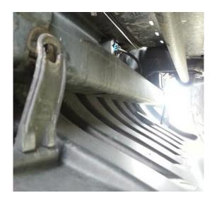
B) Remove the factory front bumper by re-moving the 4 factory nuts on both bumper mounts.
