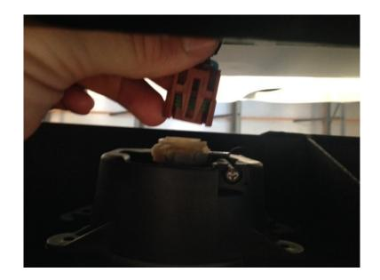
Note: For LFS Series bumpers cut the factory fog light harness off and splice the wires coming from your bumper into the factory fog light wiring.
