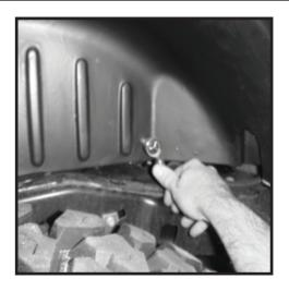
5. Secure the axle vent hose with the Wheel Liner mounting hardware on the rear passenger side. There is a hole in the plastic clip attached to the hose for making the attachment. The hose should be secured to the rear most mounting hole in the Wheel Liner just above the frame rail.
