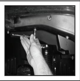
4. If Flat Flares were previously installed, remove all bolts securing the rear Flat Flare except for the top 2 bolts. Position Wheel Liner and loosely install Push Rivets. Using the supplied M6 hardware, loosely fasten the wheel liner to the vehicle using the mounting locations provided in the Wheel Liner. Once all holes are lined up, fully engage push rivets and tighten all bolts. NOTICE: Do not overtighten bolts as this could cause damage to the Liners.
