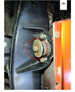
bolts from the vehicle. Using a 18mm socket remove the body mount
