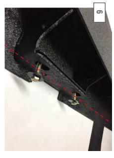
Using the handle on the plate-nut align the plate to the pinch weld holes. Using the supplied bolts and washers secure them to the pinch welds. Then fully tighten the body mount bolts. The dotted red line above represents the pinch weld.
