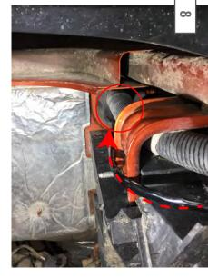
Run the switch wiring harness through the battery box into the inner fender, then carefully punch a hole through the body grommet feed the plug into the passenger compartment.
