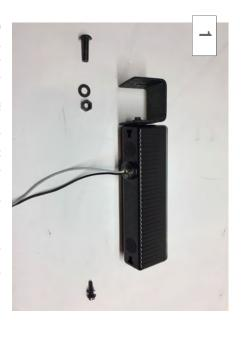
front LED light. Repeat this for all (4) lights. faces the tire. Pictured above is the passenger come threaded into the light. \*\*Note: The spacer the LED light using the small phillips scres that Begin by installing the U-shaped spacer bracket to
