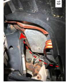
Run the shorter wires down through the battery box down to the passenger side LED lights. Connect the wiring to the LED lights.
