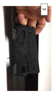
more clearance please add the supplied bracket spacers to provide Note: If sliders contact the vehicle after installation, Place the plate-nut brackets into the slider. The handle will be used to align the plate in step 6.
