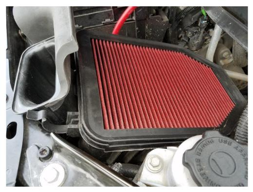
6. Place the top back on the air box making sure it gets a good seal all the way around. It can help to start by seating the right side first then working your way toward the air inlet. Now connect the 4 metal clips around the air box. Install the 2 bolts removed with a 10mm socket, but be careful not to overtighten. Then reinstall the engine cover if removed.
