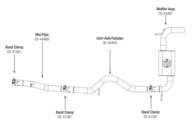
**Step 1:** (Read Instructions prior to installation) Remove your stock exhaust from the rear of your truck working your way forward. Take caution not to damage the factory isolation mounts as they will be reused. It may be helpful to lubricate the isolation mounts prior to disassembly. It is recommended to not fully tighten the clamps until the entire system has been installed.
