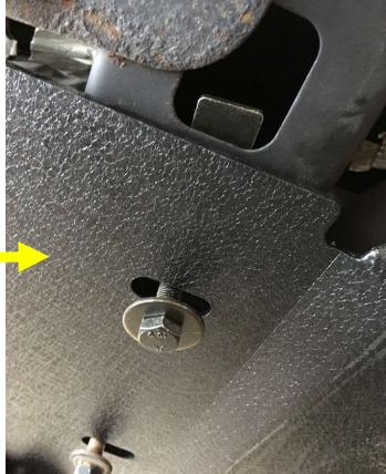
7. Torque all 6 bolts to the proper spec using 18mm & 19mm wrenches (i.e. ½" hardware to 90 ft-lbs).
