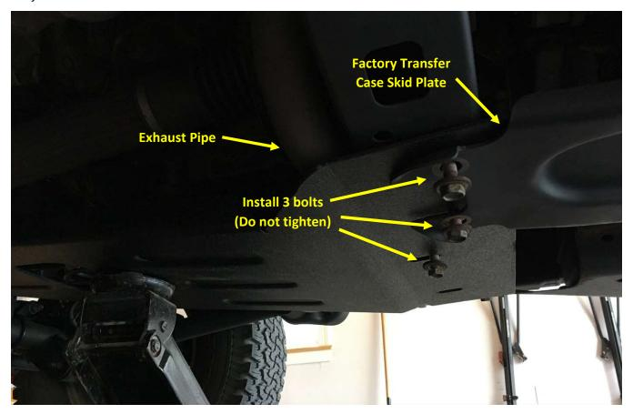
Note: If using the factory transfer case skid plate, interference may be present at the formed gusset on the passenger side with the new transmission skid plate. Cut the corner of the gusset off to allow the transfer case skid plate to sit flush against the transmission skid plate. This interference may not occur on all models/years.
