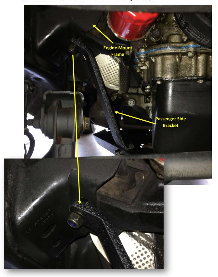
4. Similarly, install the driver side transmission skid plate bracket between an existing hole in the engine mount frame and the driver side hole in the front of the transmission skid plate. Use a ½"x1" bolt, 2 washers & locking nut for each connection. Install the bolts but do not fully tighten at this time.
