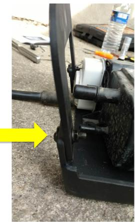
5. Using the screws, washers, and nuts that came with the kit, fasten the front bracket onto the INSIDE of the skid plate with the nut facing out. Put the washer on the screw first, then put the screw through the hole and with the nut so it looks like this. Do not tighten all the way. (Note the direction of the screw head is facing in and the nuts are out)
