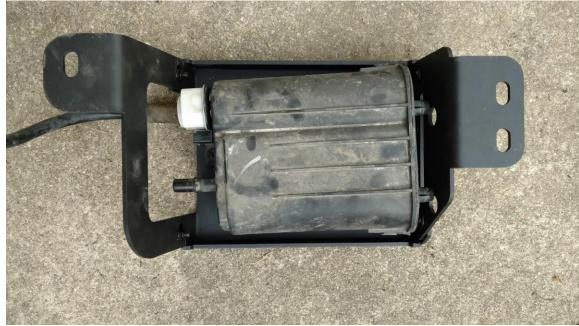
7. Place the evap canister into the fully assembled skid plate and assuming everything fits correctly, tighten the four bolts connecting the brackets to the skid plate using the 4 mm allen wrench and a 10 mm box wrench.
