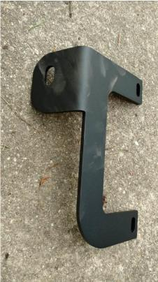
3. The bracket that will go on the front side of the skid plate has two holes in the top.
