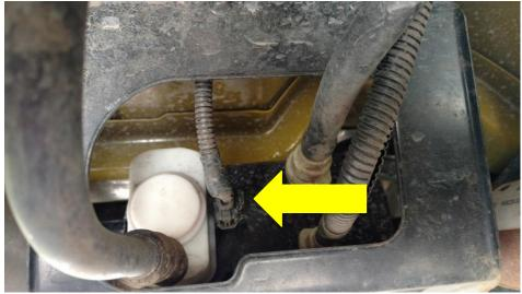
4. Disconnect the two hoses to the right by very carefully using a flat screw driver to loosen the "teeth" and then pull the "horseshoe" shaped retaining clip out. The top clip comes out to the left as shown here.
