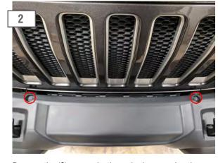
Remove the (2) upper plastic push pins securing the plastic cover to the frame rails.
