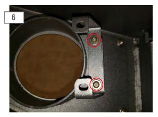
Install the (2) LED fog light brackets to the fog light mounts of the bumper using the (4) M6 torx bolts, washers, and nuts.
