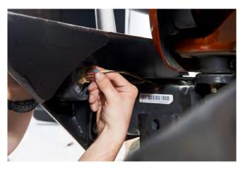
$\mbox{\bf STEP 8}$  // In most cases, the fog light harness will need to be extended. Cut and splice the wires to the appropriate length.
