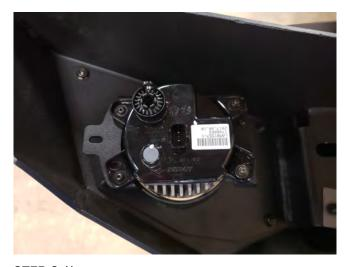
**STEP 6** // Using the supplied screws, secure the fog light housing to the bumper.
