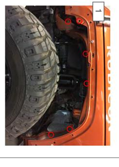
Locate the mounting locations on the fender well.
