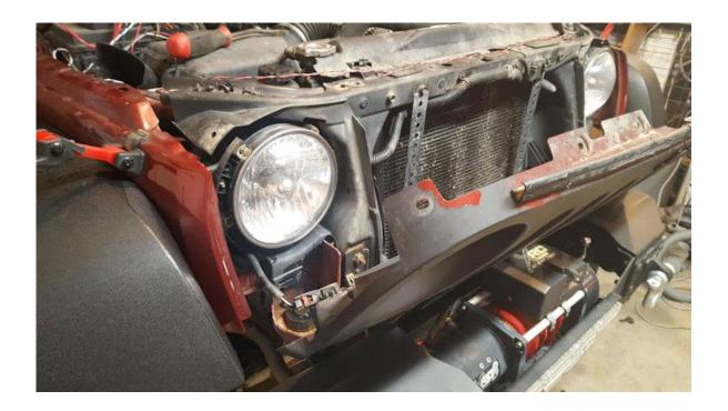
• **Step 3** Remove four T15 screws from each of the headlight trim rings. Pull out headlights to access stock bulbs and harnesses.
