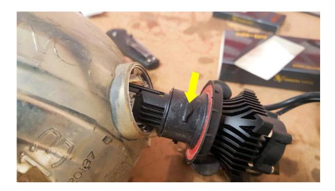
• **Step 6** Mount the Delta LED Driver in a position that will maintain enough space for the larger LED units behing the reflectors.
