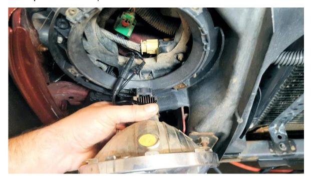
• **Step 9** Reinstall reflectors with trim rings using the stock T15 screws.
