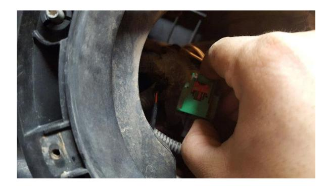
• Step 8 Connect the LED power and fan connectors from the Delta driver to the LED unit.
