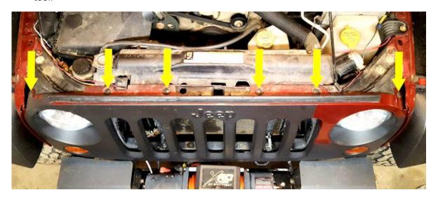
Step 2 Disconnect tabs on bottom edge of grill by pulling sharply. Tip grill forward to access headlights. You can stop here, or for easier access, unplug turn signals and remove grill completly.
