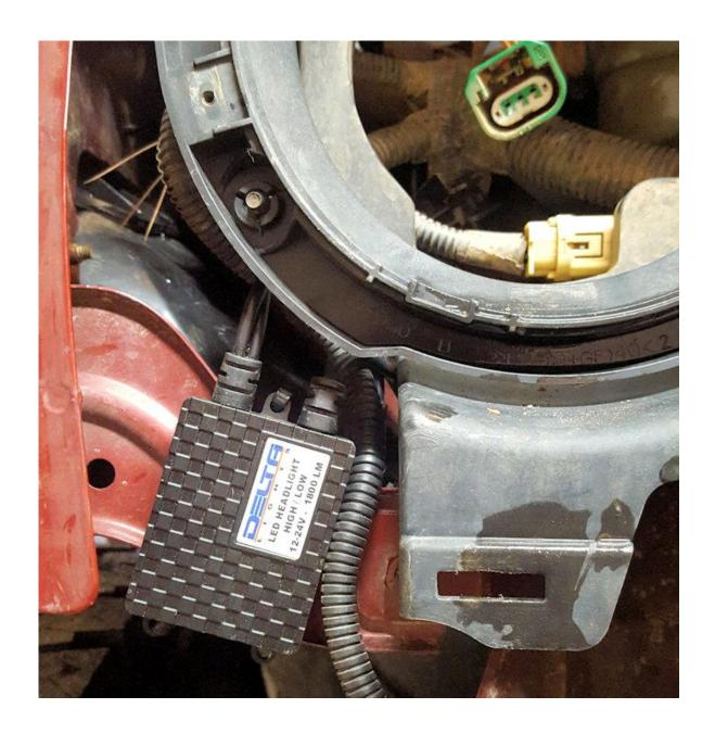
• **Step 7** Push the harness connection into the stock bulb connector. The connectors in this '09 would not snap together without trimming a small amount of plastic from the catch on the Delta harness. Rengage red locking tab.
