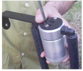
4. Locate the 8mm bolt indicated below and remove, using the ratchet and 8mm socket.
