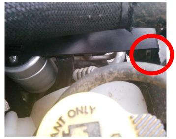
6. Remove rubber angled connection from PCV tubing on the passenger side.
