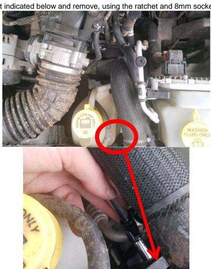
5. Install the bracket (with oil separator already attached) to the hole, and fasten back together with the removed 8mm bolt.
