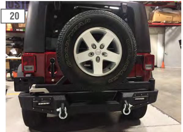
Install the spare tire using the supplied lug nuts. torque to factory spec (40-80ftlbs).
