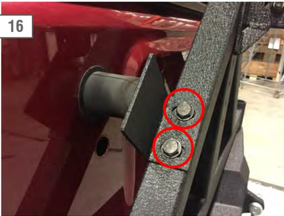
Install the tire carrier bump stop brackets using the long M12x1.75 bolts, washers, and lock nuts.
