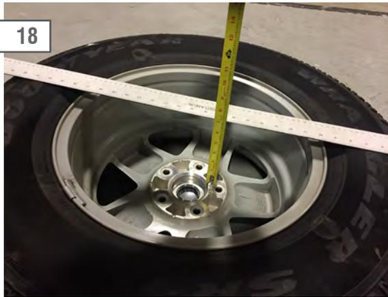
Measure the spare tire to set the hub mount spacing on the tire carrier. Place a straight edge across the tire and measure from the hub of the wheel to the straight edge, then subtract .25". (ex. measures 7.00", minus .25", hub spacing should equal 6.75").
