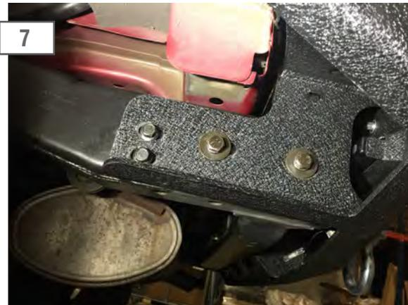
Loosely install the bumper to the frame rails using (4) M10x1.5 flange bolts and the (4) M12x1.75mm bolts, locking washers, and large flat washers.
