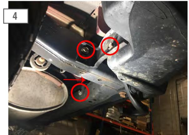
Remove the (4) 15mm bolts on the outside of each frame rail. Then remove the (4) 15mm bolts securing the plastic bumper to the frame.
