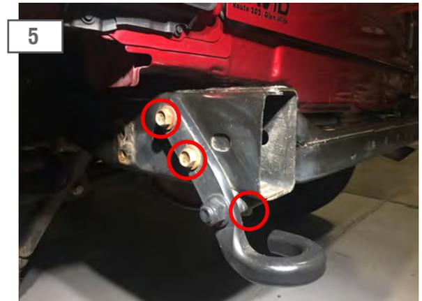
Remove the (3) bolts securing the tow hook to the driver side frame rail.
