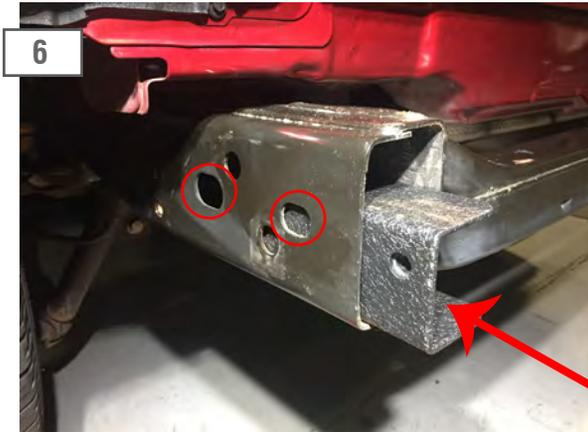
Slide the supplied bumper mount bracket into the frame rail so that the threads are visible through the (2) holes circled above.
