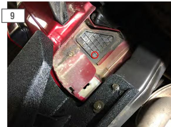
Wire the bumper mounted LED lights together and then to the reverse lights using the supplied wiring. Drill a small hole through the passenger side plastic wheel well panel and feed the wires up to the tail light. \*\*Note: There may be foam above the plastic panel, use a long screwdriver to poke a hole through it.
