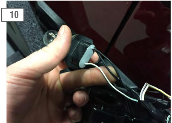
The gray wire gets wired to 12V+ and the black wire gets wired to ground. With a helper and a test light, with the engine off put the vehicle in reverse, using a test light determine which wire is the 12V+ for the reverse light. Wire the bumper lights into the 12V+ for the reverse light and a suitable ground. Ziptie any extra wire out of the way.
