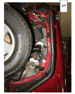
proper bolt hole alignment. M8x1.25 25mm long Allen bolts, install the forward most (5) bolts first. \*\*Note: Loosely install all Install the Barricade Flat Fenders using the supplied hardware before fully tightening bolts to ensure
