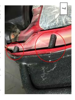
Install the supplied spacers between the inner and outer fenders using the M8x1.25 120mm bolt for the long spacer and the M8x1.25 65mm bolt for the shorter spacer.
