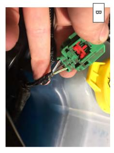
Located the headlight wiring harness, with the low beam headlight switched on, use a test light determine which wire is the 12v+ and which is the Ground. Using wire connectors, to splice the LED wiring leads to the appropriate wires in the head light wiring harness.
