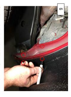
Clearly mark the holes for drilling. Remove the fender for ease of drilling. Using an 11/32" drill bit, carefully drill the (2) rear most holes on the front fenders. \*\*Note: Keep the drill level, drill through both the outer and inner fender.
