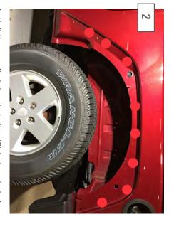
Install the supplied rivnuts in the (8) holes circled above. Begin by drilling the rivnut holes to 23/64".
