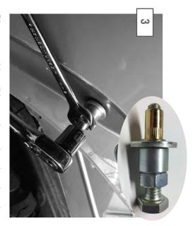
Rivnuts provide solid mounting point when there is no access behind the mounting surface. Insert the rivnut into the pre-drilled hole. Thread the rivnut tool onto the rivnut. Using a 16mm wrench, hold the nut in place while turning the head of the bolt with a 17mm ratchet. Tightening the bolt will clamp the rivnut against the sheet metal. \*\*Note: Do not over tighten the rivnut. Doing so can pull the threads out of the insert.
