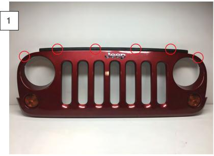
Using a panel removal tool, remove the (6) push clips holding the grille cover to the vehicle. Unplug the turn signals and pull grille cover from the vehicle.
