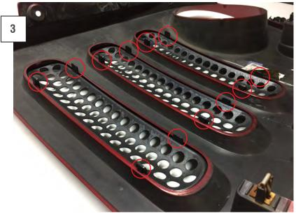
Press the insert into the grille cover ensuring that the insert clips onto the back edge of the grille. Install all (7) inserts and then reinstall the grille in reverse order.
