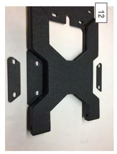
Place the thin spacer behind the upper tire carrier bracket mount, and the thick bracket behind the lower tire carrier bracket mount.
