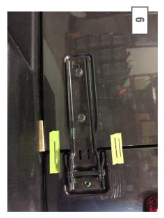
Shim the bottom of the tailgate to prevent it from sagging when the hinge bolts are removed.
