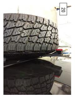
Place the 3rd brake light in the bracket. With the tire mounted, set the brake light height. Tighten the upper and lower brackets together. Then, secure the factory 3rd brake light in the bracket using the factory screws.
