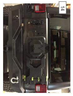
Mount the tire carrier base to the tire barrier bracket using the (4) provided bolts and washers.
