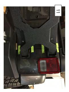
Install the tire carrier bracket to the hinges using the supplied hinge pins. Once installed secure the hinge pins using the provided c-clips. \*\*Note: A rubber mallet may be needed to seat the hinge pins.
