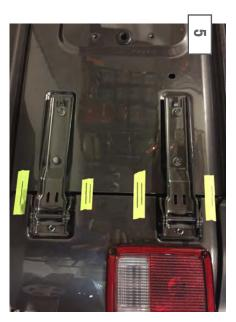
blade to cut the tape in half at the seam. tailgate in several locations. Use a straight edge to can line up the tailgate correctly if need. Mark the Next, apply painters tape to the vehicle so that you mark the tape as a visual reference. Use a razor
