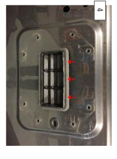
vent. Using a panel removal tool, remove the factory air
