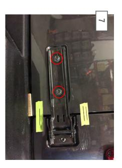
Remove the plastic hinge covers followed by (2) 13mm bolts securing the hinge each hinge to the tailgate.
