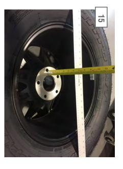
Next, loosely install the tire carrier. Measure the backspacing required by placing a straight edge across the tire. Then, measure to the mounting hub of the tire.
