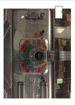
grommet to remove the plug from the vehicle. Remove the (8) 13mm bolts holding the factory tire carrier in place. Remove the 3rd brake light wiring
