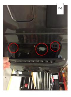
Close the tailgate. Do not install the vent cover. removal tool. Unclip the brake light wiring harness. connector. Remove the vent cover with a panel Open the tailgate to access the 3rd brake light
