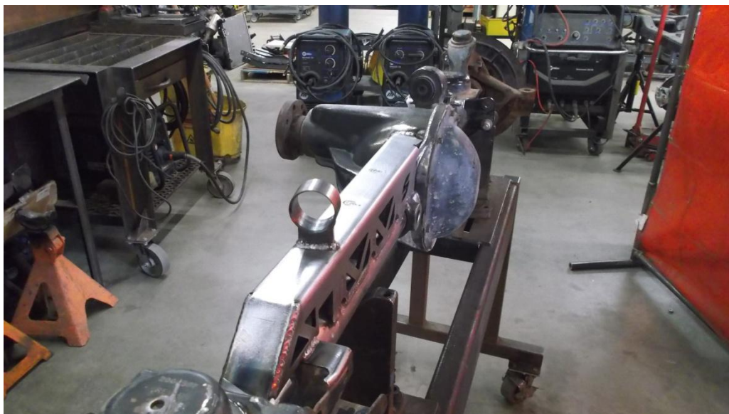
Figure 19. Bushing Mount Welded to Truss
