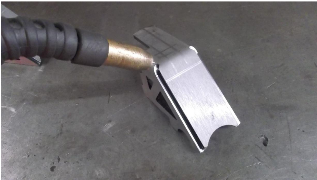
Figure 7. Welding Truss Bend Seams
