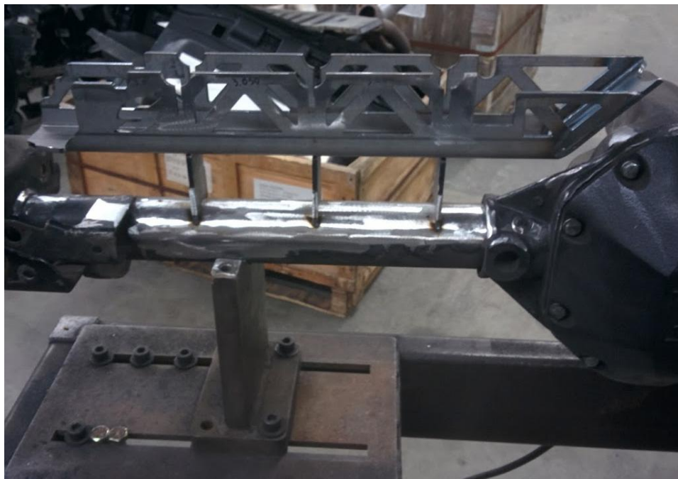
Figure 11. Truss Used as a Fixture
