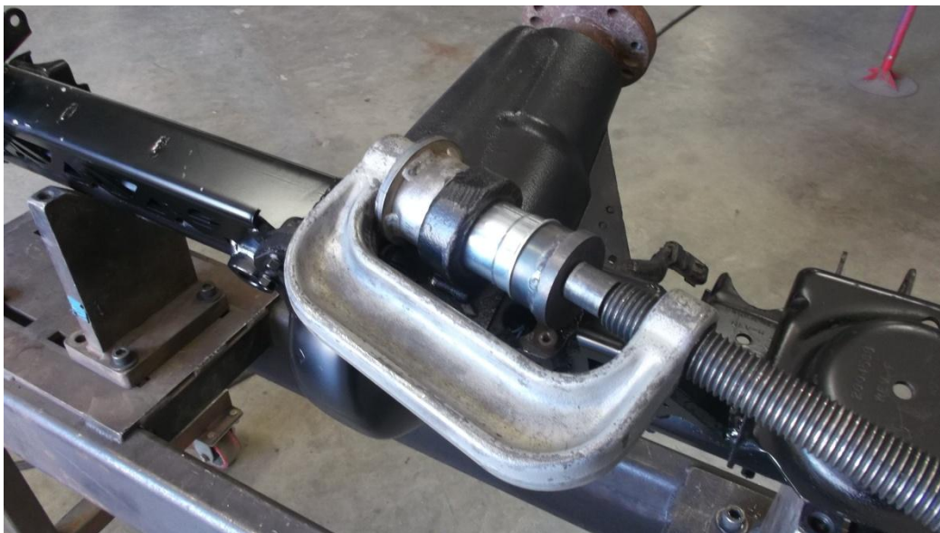
Figure 21. Installing Upper Control Arm Bushing with Ball Joint Press
