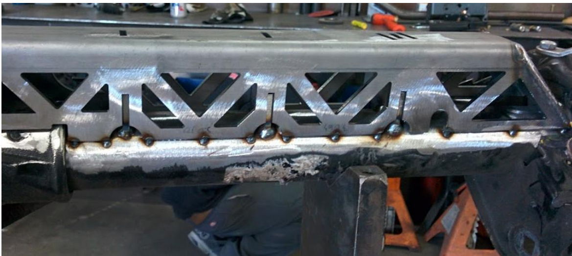
Figure 13. Back side of Truss Tacked
