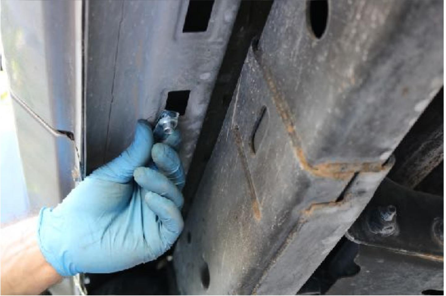
9. With the Nerf Step in place, proceed to secure all bolts. Using a 13mm socket wrench for the lower bracket bolts and a 1/2 wrench for the top bracket bolts.
