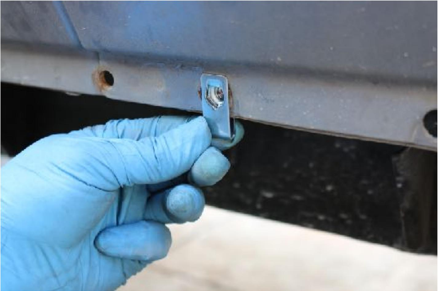
7. Position Nerf Step against pinch weld and attach the top bracket to the Clip Nut. (Do not tighten fully at this point)
