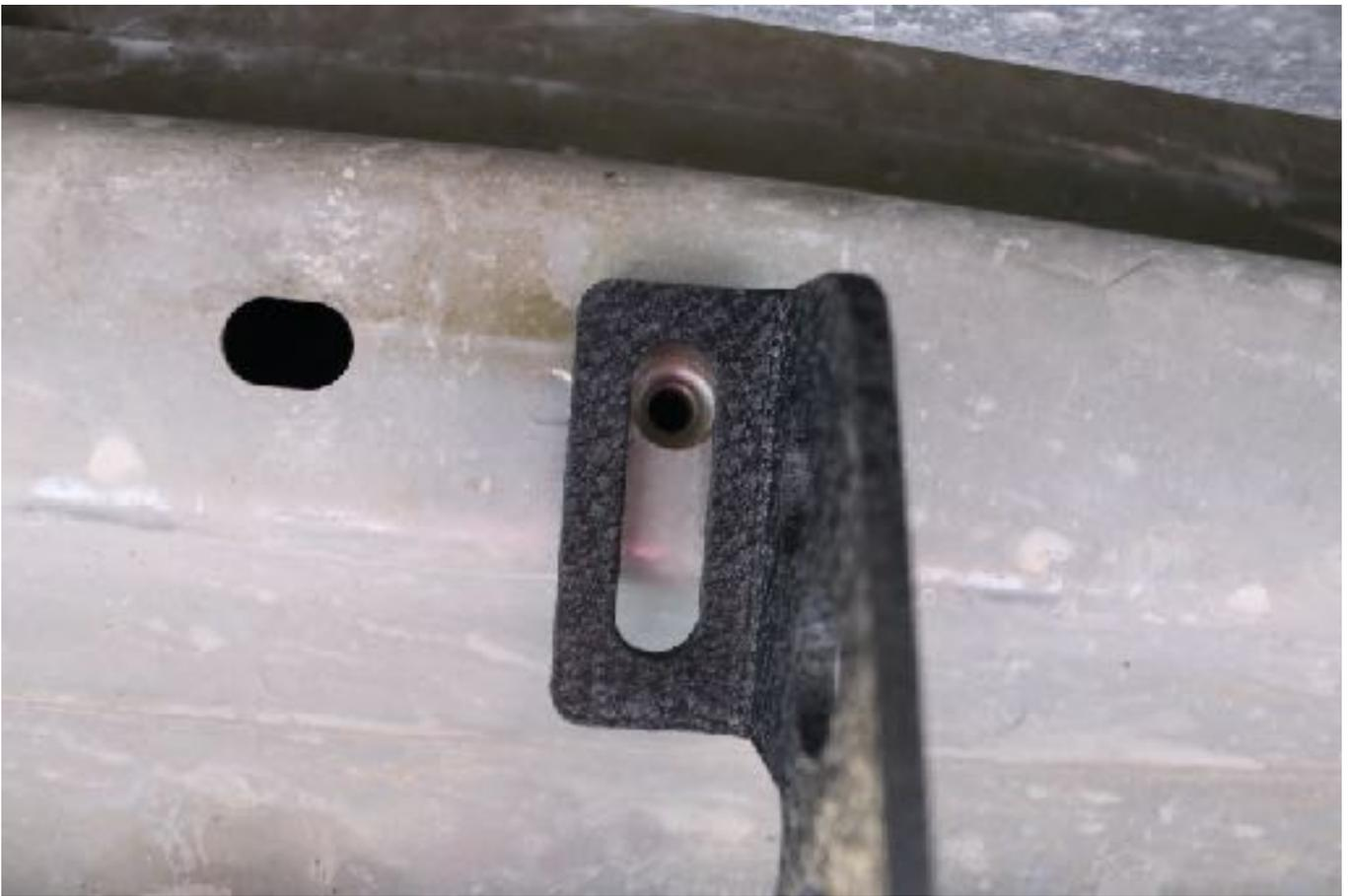
4. The top brackets should line up with the holes in the pinch weld. In some cases these holes will need to be drilled. Identify and mark these holes.
