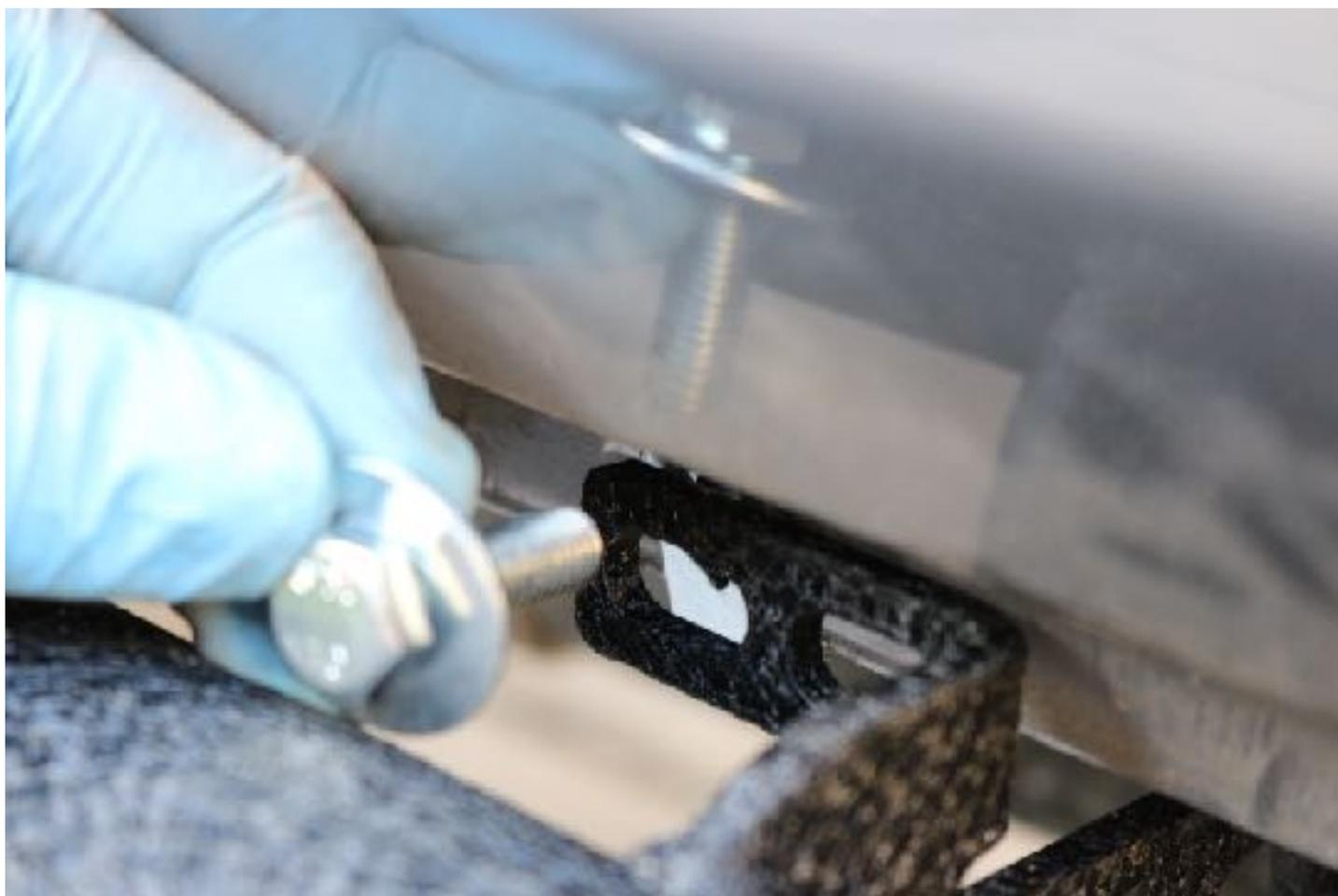
8. If the lower bracket lined up with the pre-existing holes under the Jeep body as shown in Step 3. Bolt these down using the provided hardware. In some cases, the lower bracket will not line up with the pre-existing holes, in this case you will need to place a Clip Nut into the holes positioned on the underside of the Jeep body.
