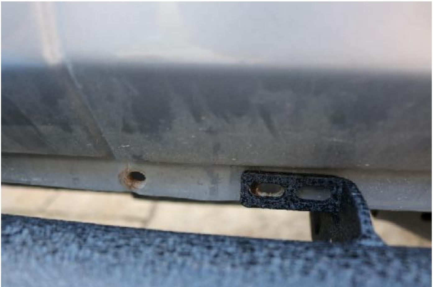
5. Drill marked holes with with 3/8” Drill bit. (Make sure to paint drill holes after to reduce the risk of rusting)
