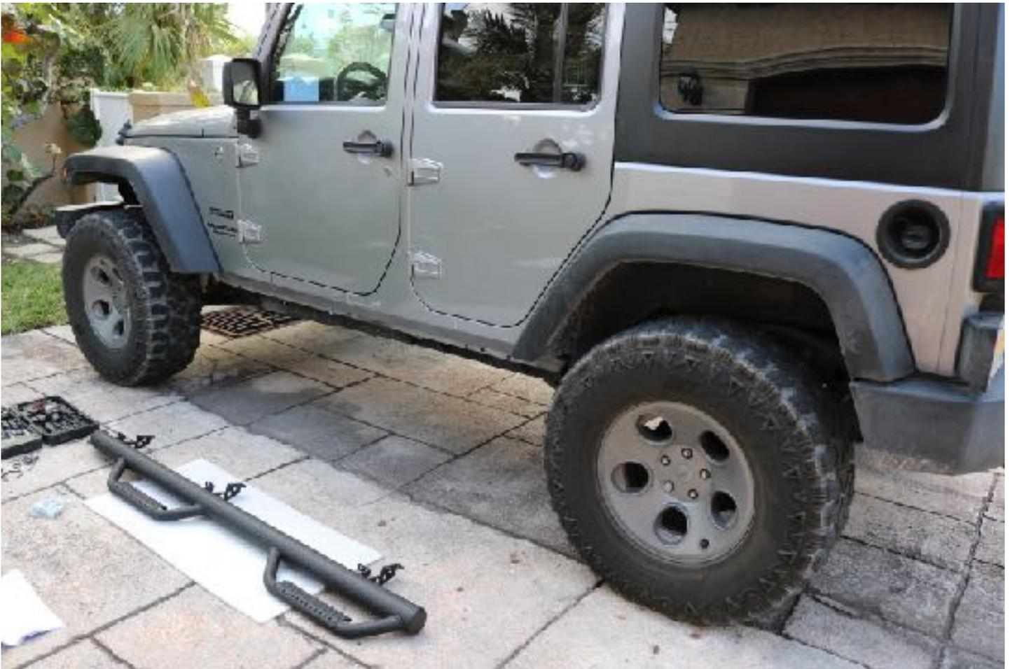
2. Remove Factory Running Boards if necessary. (This can be done by removing the three 13mm bolts facing upwards and the six 10mm bolts facing outwards on each running board)
