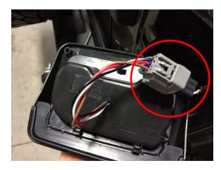
Step 4: Install the Raxiom tail light with the factory screws. Reconnect the battery terminal and ensure the tail light functions properly.
