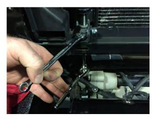
Step 6: Loosely attached the lower light bracket using the supplied 1/4" bolt, washers, and nuts.
