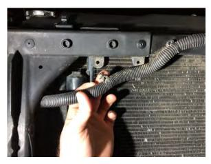
Step 7: Remove the wire loom clips from the upper radiator support.
