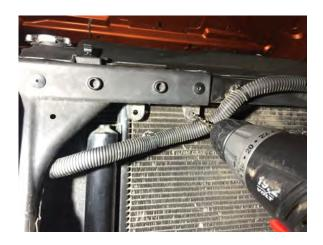
Step 8: If necessary, carefully drill the existing upper radiator support holes to 9/32".
