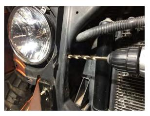
Step 4: Drill the (4) exsisting holes to a 23/64" diameter.
