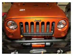
Step 10: Reinstall all grille clips and turn signal plugs.
