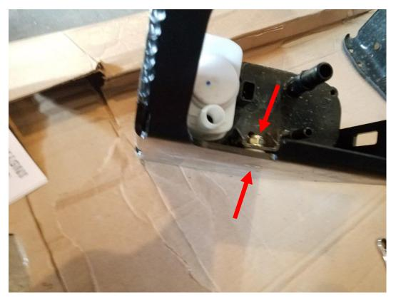
**11.** Next, install the skid plate using the 3 factory bolts removed in step 5. Make sure the front bolts go through the skid plate and the front evap mount bracket. Tighten the bolts using a 16mm wrench for the front 2 bolts and a 16mm socket for the rear bolt.
