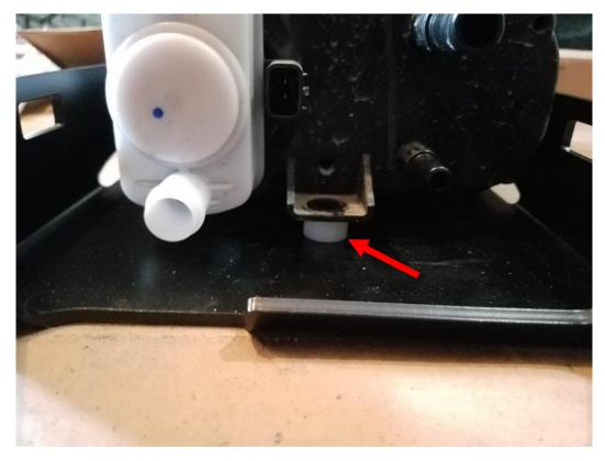
**9.** Slide the evap canister forward until the front bracket holes line up with the skid plate holes. Make sure the bracket is below the skid as shown below. The rear mount hole should line up close to the skid hole. It doesn't need to be perfect, but it needs to be close.
