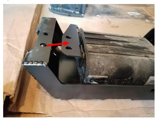
8. Next, install the supplied nylon spacer under that rear mount of the evap housing.
