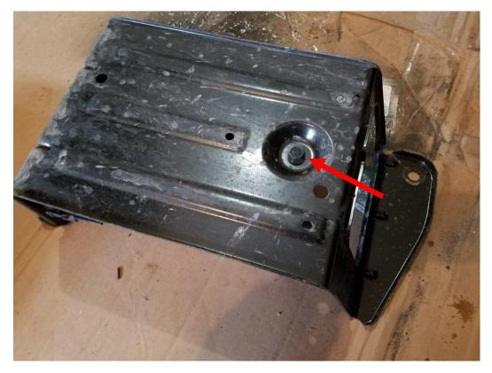
7. Place the evap canister into the new skid plate oriented as shown. Then install the supplied 2012+ bracket as shown below. It will slide over the 2 plastic pieces that stick out the front upper side of the evap housing. You will need to push this bracket as far onto the housing as possible. You can use a rubber mallet to gently tap it down into place.
