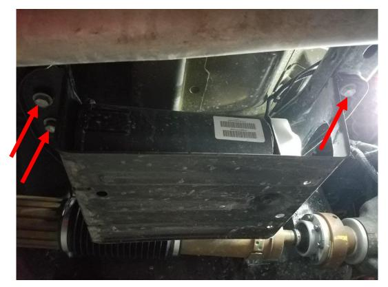
6. Using a 13mm socket and 13mm wrench, remove the bolt holding the evap canister to the bracket.
