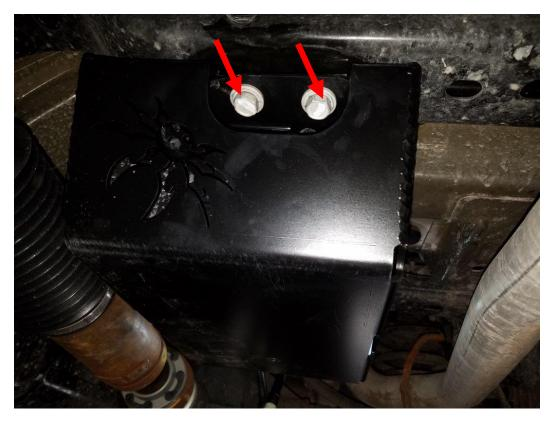
**12.** Tighten the rear evap canister bolt using a 3/16" hex key, and 1/2" wrench.
