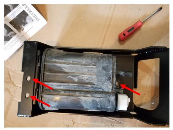
**10.** Then insert the supplied flat head cap screw into the countersunk hole on the bottom of the skid plate, through the nylon spacer and the evap mount. Use the supplied washer and lock nut, and only hand tighten for now.
