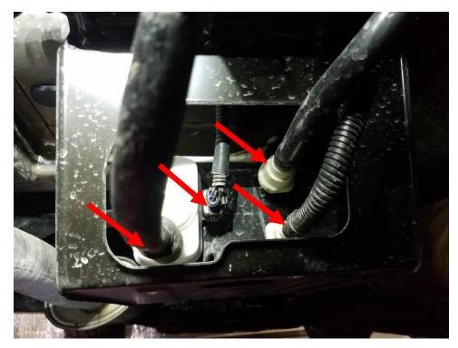
**3.** Looking from the side you can see the 2 small tabs that you will need to press in. You can use needle nose pliers or a flat head screwdriver to push them in. Be careful as these plastic pieces break easily. Both hoses can be removed the same way. Note: If you break these pieces you can find a suitable replacement at an auto parts store in a retaining clip assortment. You could also use a small zip tie.
