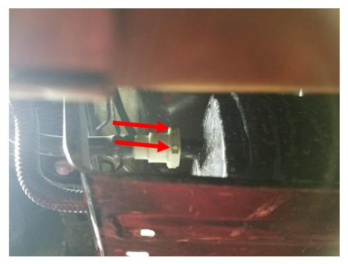
**4.** This is what the connector will look like then it is ready for removal. Once you have this piece out, you can pull the hose off the evap canister. Do the same to remove the lower right hose.
