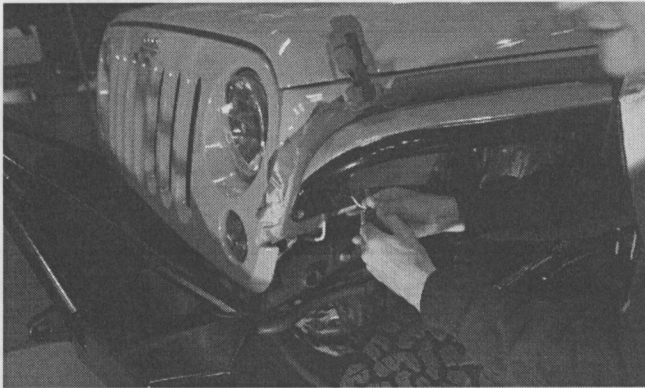
14. Unbolt and remove the Crusher Flare.
