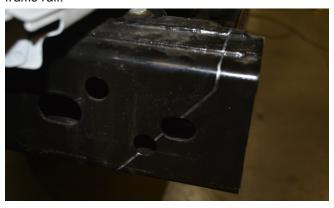
7. Use a torch, plasma cutter, pneumatic or electric cutoff wheel, reciprocating saw, or the cutting device of your choice to cut the outboard, top and bottom surfaces of each frame rail along the cut-lines made in the previous steps.
