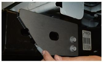
5. Continue marking the cut-line over the top surface of the frame rail. Use a square to ensure that the cut-line is exactly perpendicular to the outer edge of the frame rail. Use the same technique to continue the cut line on the bottom of the frame rail.
