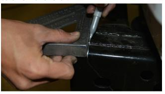
**6. Repeat the cut-line marking process** for the other frame rail.
