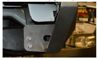
11. Insert a 3/8-16 X 1 Gr8 Hex Head Cap Screw (with 3/8 Gr8 Flat Washer) through the hole on the bottom of the BFH II Rear Bumper where it fits over the frame rail.
