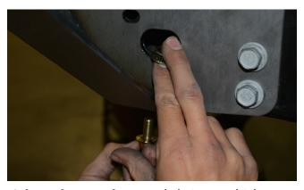
**12. Tighten the 4 OE bumper** bolts (2 per side) that were loosely installed in a previous step.
