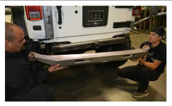
10. Re-install two of the OE bumper bolts on each side, through the holes provided on the bumper's mounting plates into the existing threaded holes in the side of the Jeep's frame rail. Do not fully tighten them yet.
