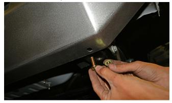
Insert a 3/8-16 Gr8 Serrated Flange Nut through the large oval hole on the side of the bumper's mount plate, and thread it on to the bolt that was inserted from below. It will be possible to hold the nut in place with a finger, but not possible to reach it with a wrench. The serrations on the bottom of the flange will work to keep the nut from spinning as the bolt is tightened with a wrench on the outside/bottom of the bumper. Install and tighten this hardware on both sides of the bumper.
