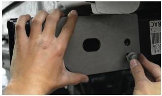
4. Use a light-colored felt-tip marker or scribe to mark a cut-line along the diagonal edge at the rearward end of the cut template.
