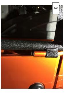
secure the door to the hinge. hinge. Use the supplied M8 nut and washer to rubber mallet to seat the door all the way onto the Install the Adventure Door, you may need to use a
