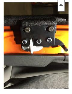
bolts, flat washers, and lock washers. Loosely install the door latch using the M8x1.25
