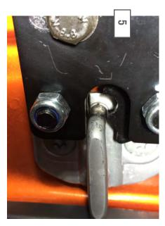
and closing the Adventure Door. the striker will result in a smooth feel when opening \*\*Note: Spending extra time aligning the latch to Align the door latch with the striker as seen above.
