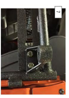
Install the mirror mount on the Adventure Door using the M10x1.5 bolt, lock washer, and flat washer.
