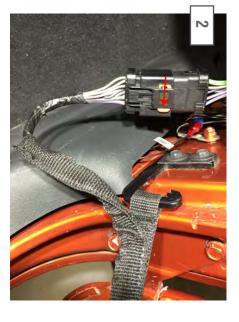
the dash. Unlock the red locking mechanism and from the vehicle. then unplug the connector. Slide the hinge strap off the door's electrical connector by tracing it under Roll down the windows so that the door is easier to the chassis mount. Lift the door up to remove it handle while removing it from the vehicle. Access
