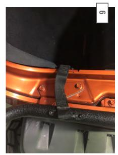
Remove the Phillips screws securing the Adventure door strap mount, install the door strap to the Adventure Door and then to the chassis mount. \*\*Note: Using the correct size philips head screw driver will prevent stripping of the screw head.
