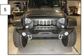
Reinstall the grille cover in reverse order, making sure to reconnect the turn signals.
