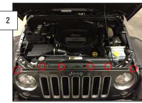
Next, raise the hood to gain access to the (6) plastic push clips securing the factory grille to the vehicle. Firmly pull on the bottom of the grille to remove the grille from the vehicle.
