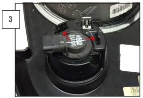
With the grille removed, depress the (2) retaining clips on the factory turn signals to remove them from the grille.
