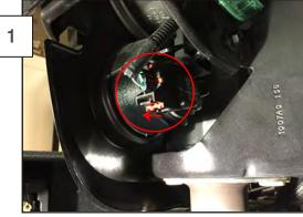
Access the connectors on the rear of the turn signals from the wheel well. The turn signal clips have a red locking tab, first slide the locking tab out. Then depress the clip to remove the signal plug.
