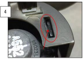
Install the factory turn signals on to the Defender Grille. \*\*Note: It may be necessary to lightly trim the grille tab to install the turn signal. Use a razor blade to trim a little bit at a time. Test fit after each trimming.
