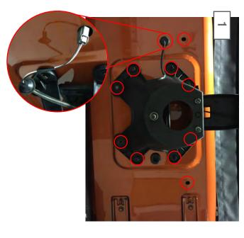
Start by removing the spare tire. Remove the rubber spare tire bumpers. Remove the 3rd brake light grommet from the vehicle and unclip the plug. Remove the (8) bolts holding the factory spare tire mount to the vehicle.
