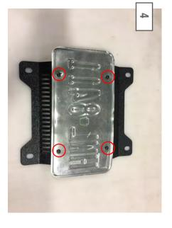
Install your license plate on the outer bracket off the car for ease of installation. Use the (4) Allen head bolts, washers and lock nuts included. \*\*Note: License plate is installed backward for photo purposes only.
