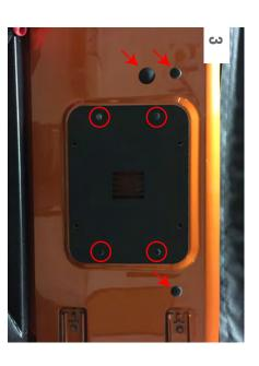
Install the Spare Tire Delete back plate by loosely installing the factory bolts in the holes circled above. Install the (2) small grommets in the factory spare tire bumper mount locations, and the large grommet where you disconnected the factory 3rd brake light.
