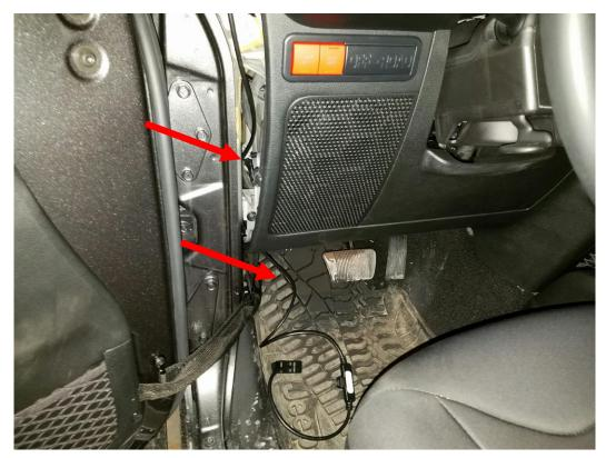
7. Using the supplied zip ties, coil the extra cable and tie it up out of the way. Use scissors to clip off the extra from the cable tie. *Note: If you will use the EAS accessories, you will attach it to the adapter in the middle of the cable.*
