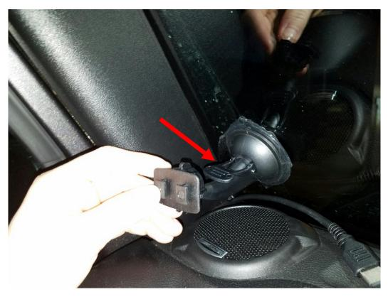
**10.** Plug the HDMI cable into the back of the TrailCal. Then align the grooves on the back with the tabs on the mounting plate and push it down into place.
