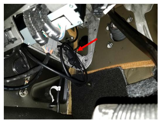
**8.** Then attach the connector to the Jeep port located above the left side of the floorboard. I also recommend using one of the supplied zip ties to hold the connector in place. Use scissors to clip off the extra cable tie.
