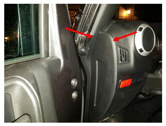
4. Using the supplied cable, feed the HDMI side through the open panel, up behind the weather stripping in the back of the dash. From the top of the dash, you can use your fingers to compress the weather stripping to easily fit the cable through.
