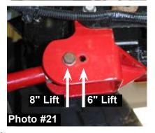
**Note:** The rear upper link brackets feature two mounting locations for the upper arms. When installing a Skyjacker 6" lift, use the forward hole in the bracket. (See Photo # 21)
