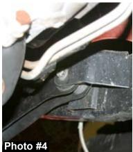
12. Attach the new Skyjacker upper control arm to the new Skyjacker bracket using the 10mm x 80mm bolt supplied. Attach the new Skyjacker upper control arm to the axle using the OEM hardware. There are four more mounting locations that attach this bracket to the frame. Two on the outside & two on the bottom. With the bracket sitting flush on the frame, drill these locations using a 9/32" drill bit. Once drilled, install the 3/8" x 1" thread cutter bolts in these locations. (See Photo # 5 & # 6)
