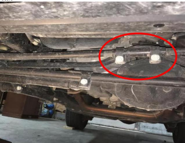
4. After removing adjusting sleeve, the short end of Drag link should still remain attached to Pitman arm
