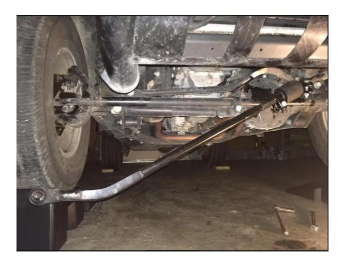
7. Make sure that both ends of drag link are equally engaged into the Griffin Attenuator.
