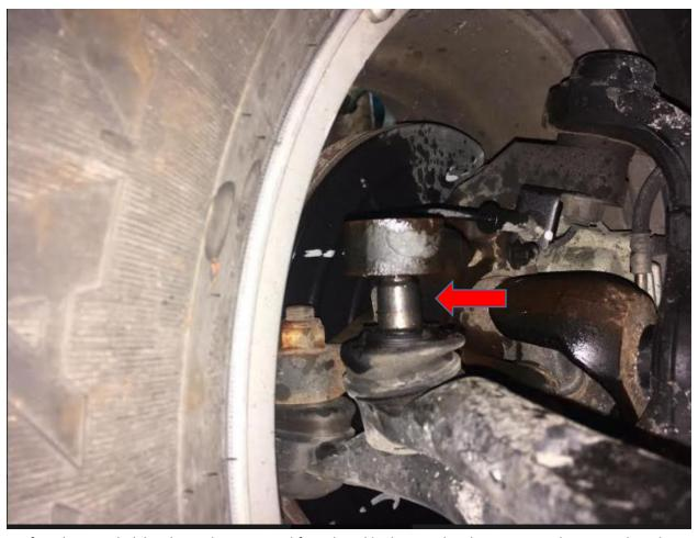
3. After the Drag link has been disconnected from knuckle, loosen the clamp nuts and remove the adjusting sleeve
