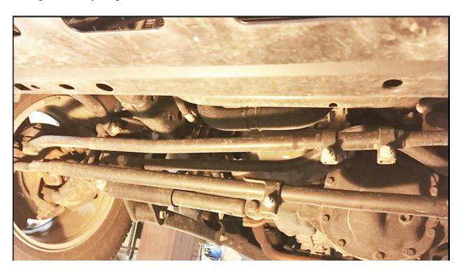
2. When the Jeep JK Wrangler is in position on lift or ramps, remove the Drag link Nut at the knuckle with 21mm wrench, which will be on the inside on passenger side wheel. After nut is removed disconnect Drag link from knuckle.
