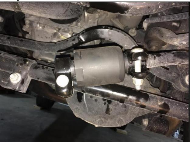
6. The Griffin Attenuator becomes the adjusting sleeve, while holding the long end of the Drag link, turn the Griffin Attenuator until the Drag link stud fits into the knuckle hole. The Drag link should be as long as it was before adding the Griffin Attenuator.
