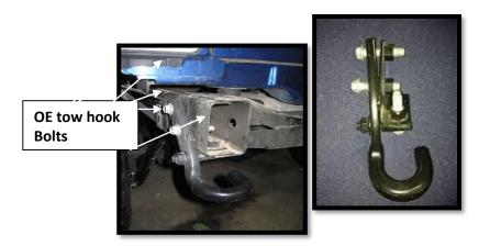
**Step 4:** Reinstall OE tow hook nut plate into inner frame rail using the bottom bolt and eyelet stud only. Make sure the nut plate aligns with the two holes in the side of frame.
