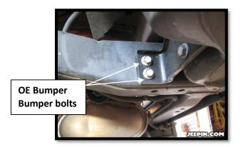
**<u>Step 2:</u>** Remove bumper. Replace OEM fasteners back into frame, these will not be used.
