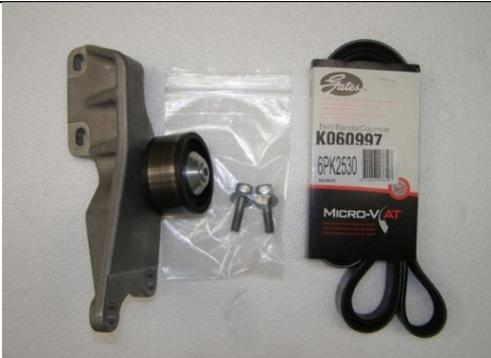
**Idler pulley bracket assembly & drive belt**
