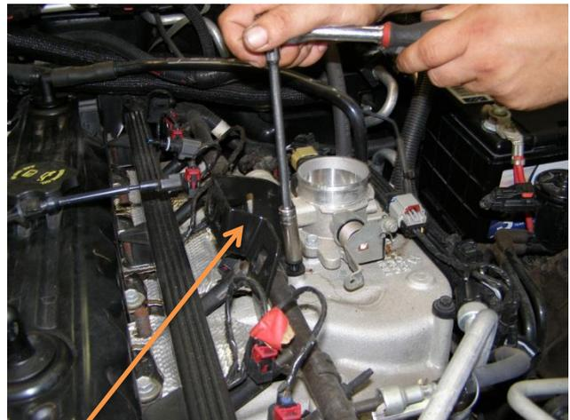
Remove throttle cable bracket
