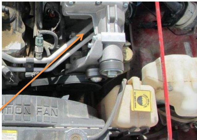
**NOTE:** Ensure that air-conditioner pipe is not damaged while trying to bend and also take special care to avoid the gas leak through the pipes and mountings.
