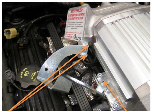
Tighten using factory M6 Hex head screws
