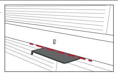
8. Flip sensor 180° from original position and reinstall using rectangular center pin.
