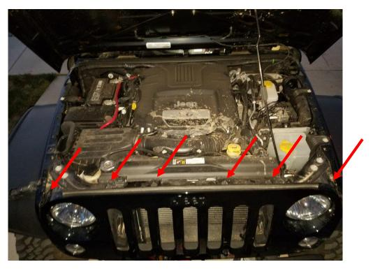
7. Use a flathead screwdriver to pull up the center piece of the retainer. This center piece can be fully removed, but save it for reinstall. Once the center piece is removed you can use the screwdriver to pry up the outer piece easily.
