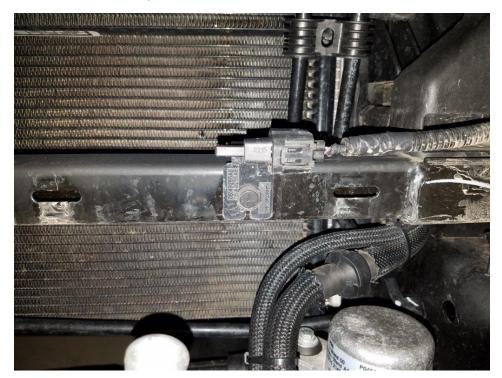
12. Rotate the sensor 180\* and reinstall as shown below. My plastic retainer broke, so I had to use a small screw instead of the center pin. You will also need to cut off the small tab that is now located on the bottom front of the sensor shown below. Use a utility knife to cut off the tab.
