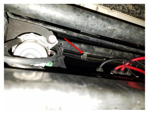
16. Now reinstall the 6 plastic retainers removed earlier. First push into place the outer plastic retainer piece as shown below, then push in the center piece. Once the center piece is pushed in the retainer should hold that joint in place.
