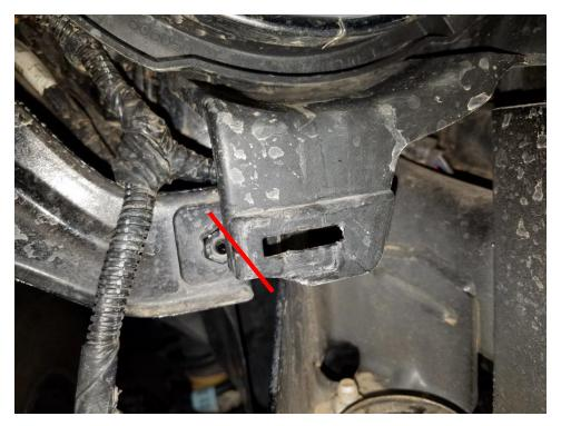
14. Now put the grille in place. Start by aligning the metal clip just behind the blinker as shown below. Push in this metal clip, then gently push in the metal clips along the bottom of the grille.
