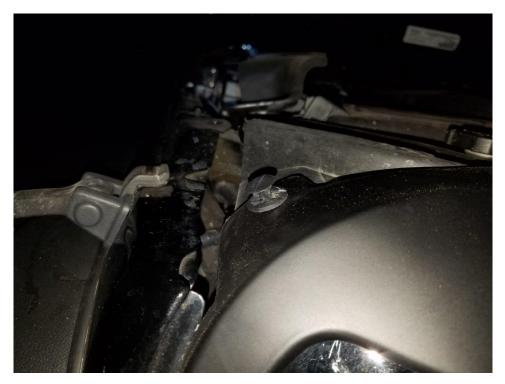
17. Reinstall both blinkers the opposite of how they were removed. Push them into place, then rotate ¼ turn upward. Do this on both sides.
