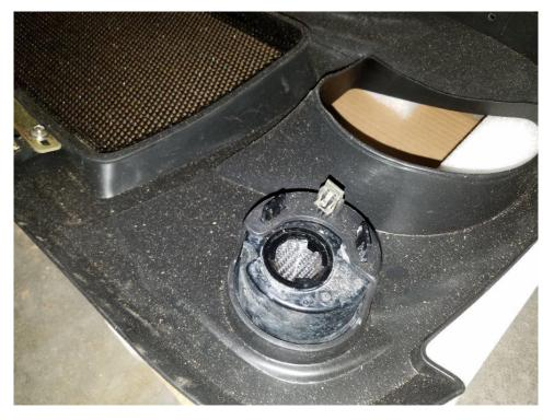
11. Remove the plastic retainer holding the ambient temperature sensor. Use a flathead screwdriver to pull out the center pin, then the sensor can be pulled off.
