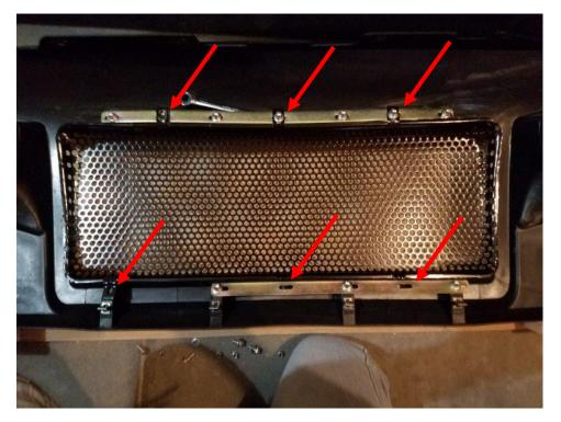
3. Then put in the star insert the same way the other one was removed. Using the same hardware that was removed, install the 6 bolts.
