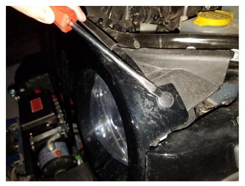
8. Once the 6 plastic retainers are removed, you can gently pull the grill forward. The remaining 6 metal clips along the bottom will pop out fairly easily.
