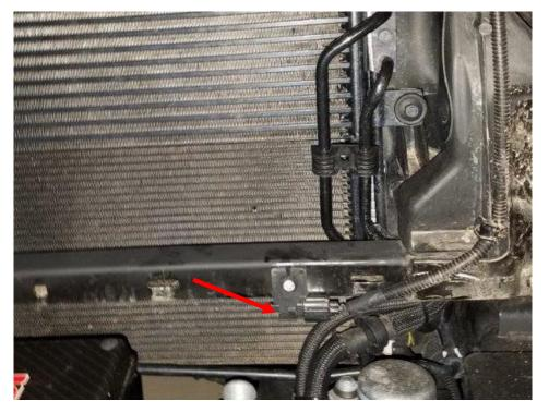
13. Using a utility knife trim the corner off the plastic bracket below the headlight as shown below. Do the same on the bracket below the opposite headlight.
