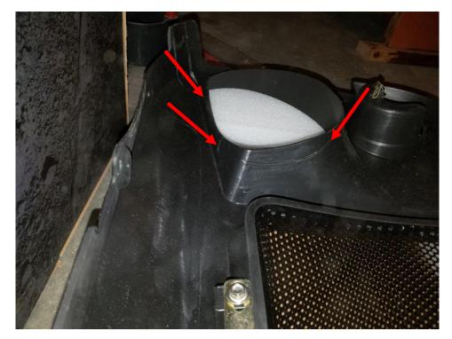
Next you will remove the stock grille. Start by removing both blinker lights. Do this by rotating the wire harness ¼ turn down as shown below the light will then pull out the back of the housing. You can leave the light connected to the wire. Remove both driver and passenger side lights.
