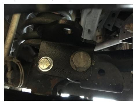
3. Install Rough Country Steering Stabilizer on axle mount and newly installed relocation bracket and tighten completely. Next, using Hydraulic Jack, lift front end of Jeep and turn driver side wheel inward.
