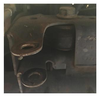
2. Install Rough Country Relocation Bracket by removing current stabilizer bracket bolt.
