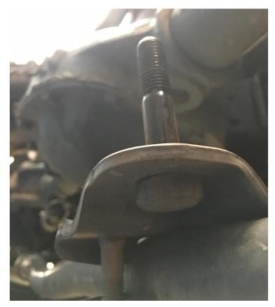
5. Complete install by installing opposite end of the Rough Country Steering Stabilizer and tighten completely.
