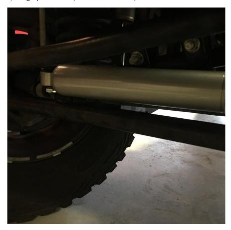
4. Loosen track bar mount and rotate 90 degrees.
