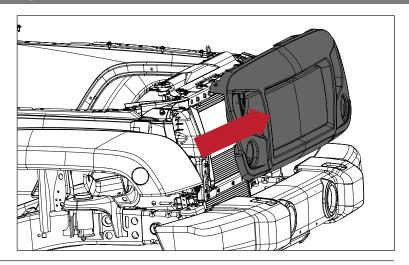
2. Remove highlighted M6 fasteners from rear of Spartan Grille. They will be reused for installing the LED insert. Remove mesh insert.
