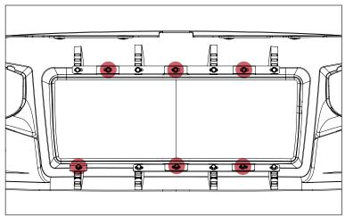
3. Install new grille insert using the M6 hardware from the previous step.
