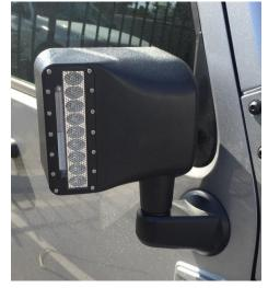
19) Wire the red and black cable in the same fashion that you would any other LED light bar. Splice the yellow cable into the positive wire of the factory turn signal light lights to use your mirrors as turn signals!
