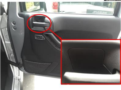
2) Remove the trim piece underneath the door handle
