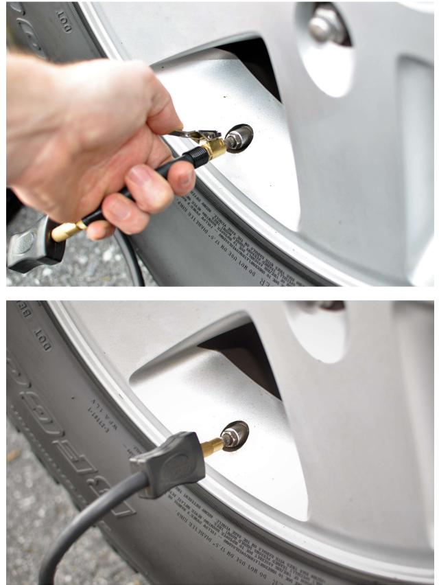
4. Turn the compressor on using the rocker switch and inflate the tire to the desired pressure. You will need to briefly turn the compressor off to get a true pressure reading of the tire pressure on the gauge.
