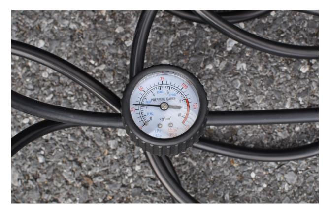
If the tire is over-inflated beyond the desired pressure, the button on the back of the gauge can be pressed to reduce the tire air pressure.
