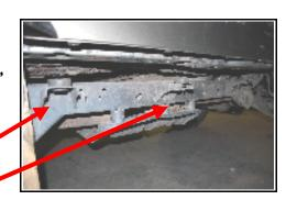
Step 7 - Place the two metal cap washers from the bushings into the two holes on the Tube Step Rocker as shown in (Figure 9). Also, place the trimmed rubber bushings back into the body mount brackets on the Jeep. Then slide the Tube Step Rocker into place onto the Jeep side while positioning the metal cap washers into the rubber bushings. Gently lower the body back down.
