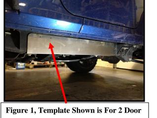
6. Before you install the Rock Slider onto your Jeep you may need to loosen more of the bolts on the gas tank skid plate and transmission skid plate in order to fit the Rock Slider Brackets in between the skid plate crossmembers and frame rail. You'll need atleast a <sup>1</sup>/<sub>4</sub>'' gap or more to make fitting in the Rock Slider Brackets much easier.
