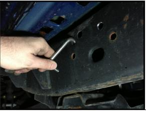
Figure 2, Install U-Bolt by inserting one leg first as shown.
