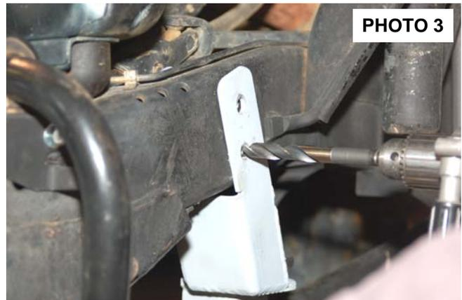
10. Remove the bracket and enlarge the outside holes only using a 29/32" bit.
