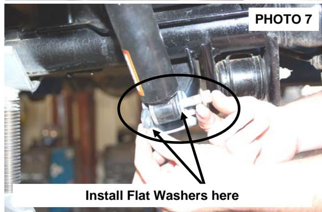
17. Install the rear Rough Country **2.2 Shock absorber Part #660576** on the upper mount and install the supplied flat washers as shown in **Photo 7** on the lower shock mounts with the factory hardware. Tighten using a 15mm & 18mm wrench. (Stock shocks shown in picture). **RCX 2.2 Series shock absorbers are designed to be installed with the piston down and body up.**
