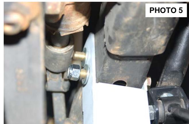
13. Remove the coil spring clip located on the bottom coil seat on the driver side of the vehicle using a 13mm wrench. Lower the axle and remove the coil spring. A coil spring or strut compressor may be needed to remove the stock coil spring.
