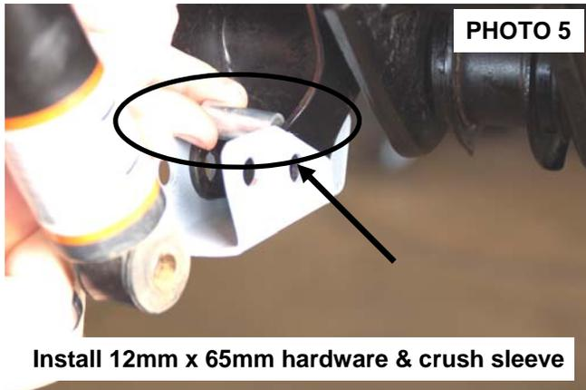
12mm bolts using a 18mm wrench & 18mm socket. Tighten the 5/16" bolts using a 13mm socket and wrench.
