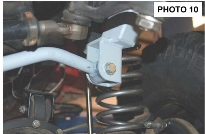
28. Install the upper sway bar mount on the top of front sway bar where the stock link was secured, using the supplied 3/8" x 1.25" bolt and washer. Tighten using a 9/16" wrench making sure the mount is straight. **See Photo 11.**
