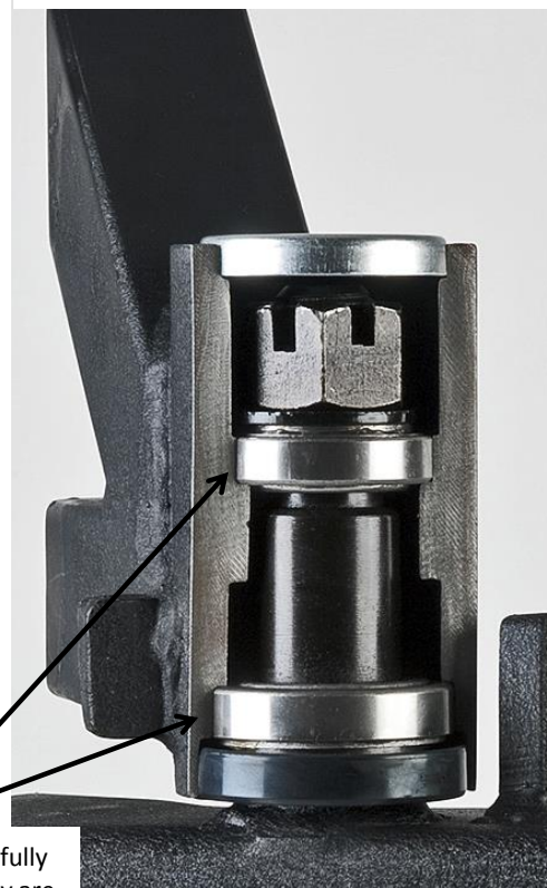
Cutaway of swing arm with bearings installed
